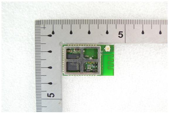
Internal View of EUT - 2 Antenna Model: RFA-02-5-F7H1-70B150
