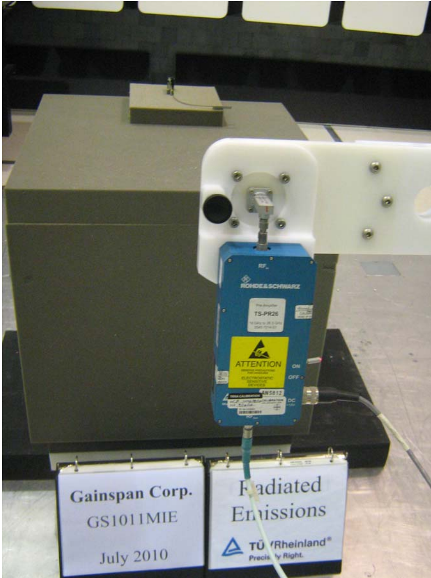
Figure 11: Test Setup with PCB Antenna for 18 GHz to 26GHz (Front View)
