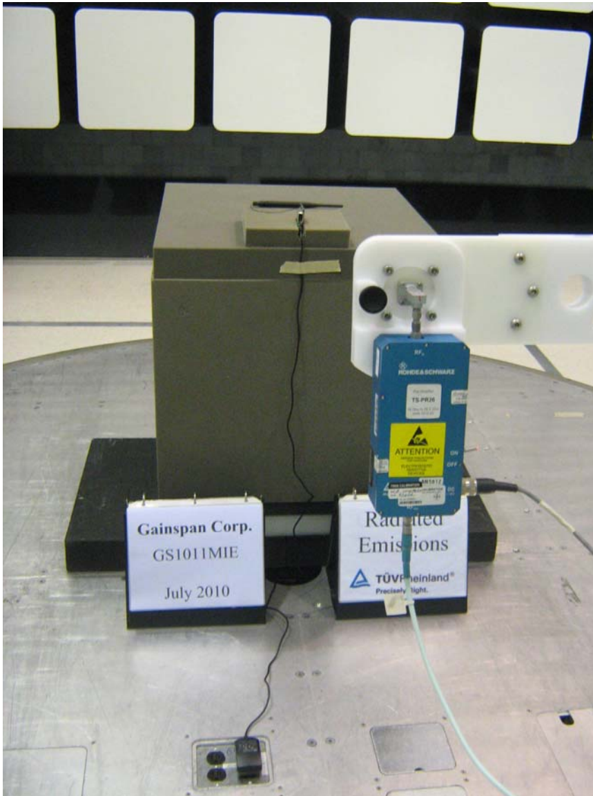
Figure 9: Test Setup with Dipole Antenna for 18 GHz to 26GHz (Front View)
