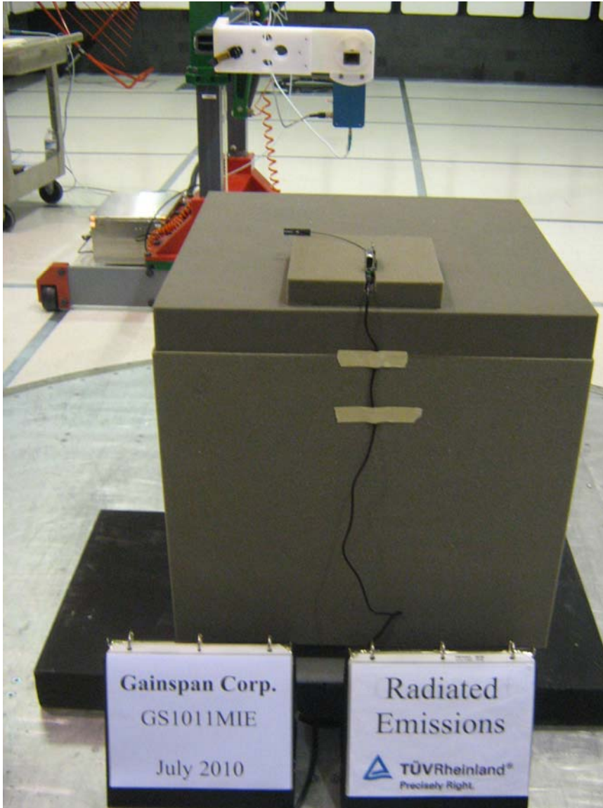
Figure 12: Test Setup with PCB Antenna for 18 GHz to 26GHz (Rear View)
