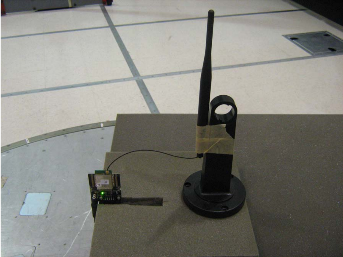
Figure 15: Radiated Emission Setup with Dipole Antenna on Z-Axis
