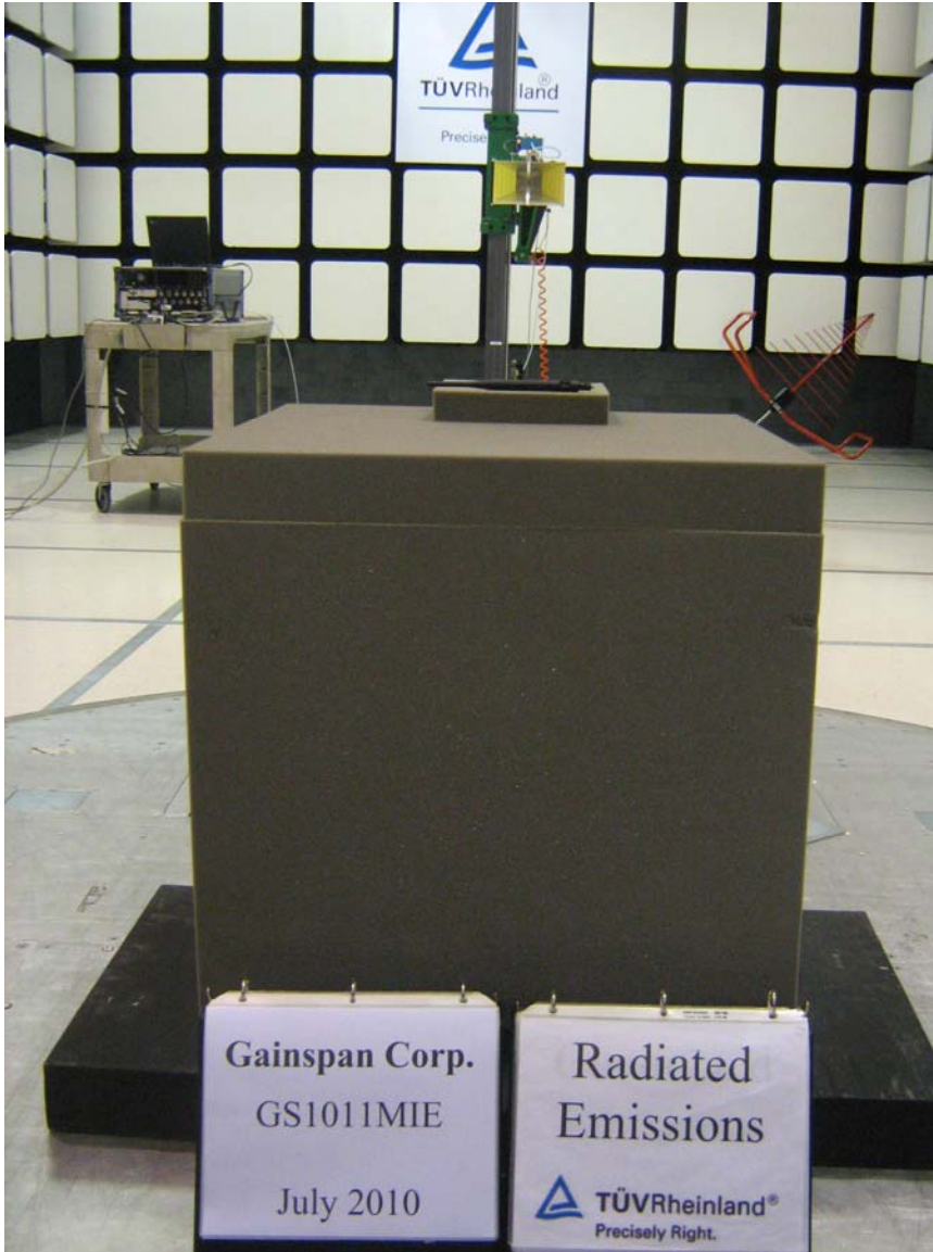
Figure 6: Test Setup with Dipole Antenna for 1GHz to 18GHz (Rear View)
