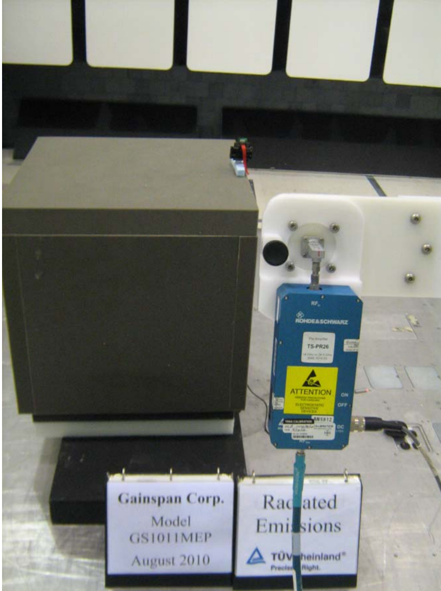
Figure 6: Radiated Emission Test Setup for 18 GHz to 26GHz (Rear View)
