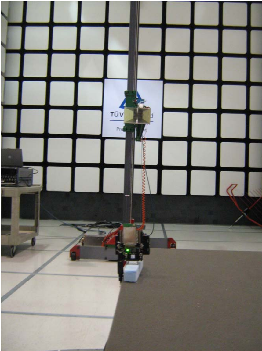
Figure 3: Radiated Emission Test Setup 1GHz to 18GHz (Front View)
