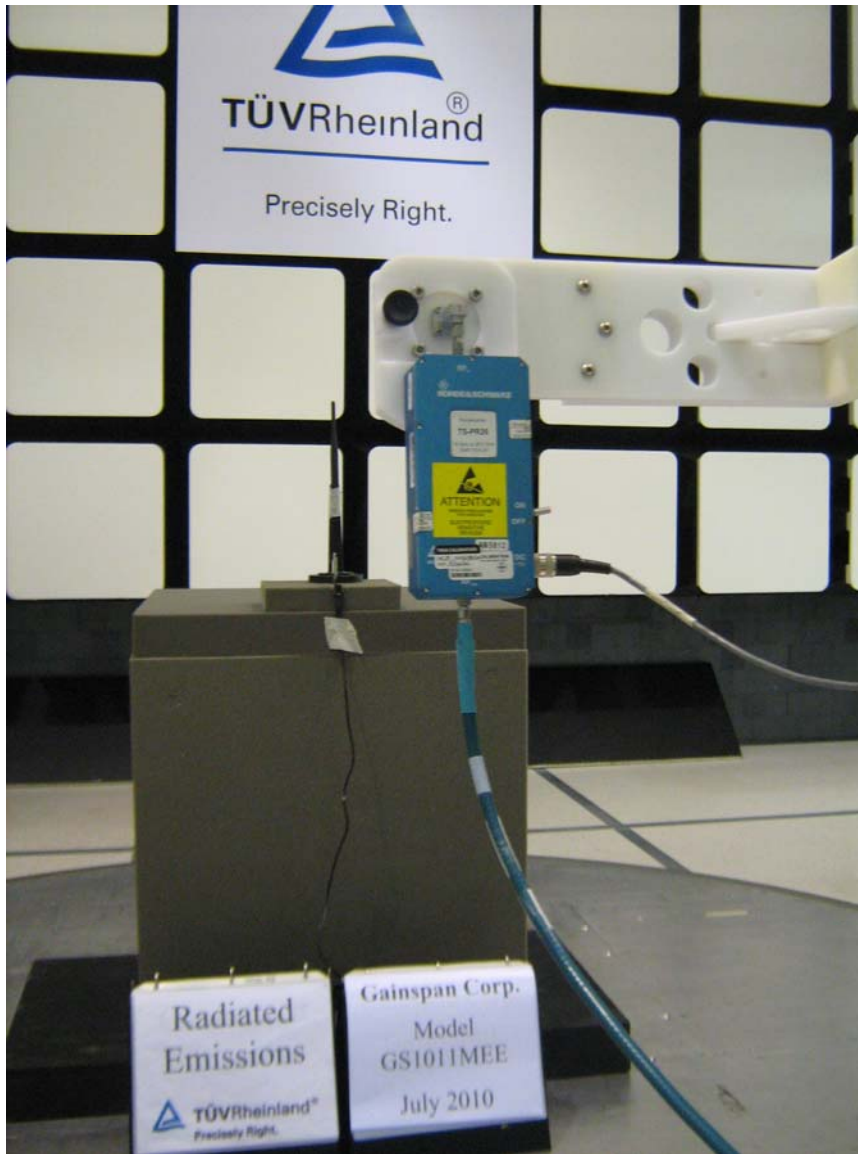
Figure 10: Test Setup with Dipole Antenna for 18 GHz to 26GHz (Rear View)
