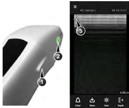
Figure 5-3. Dual probe: Orientation mark, linear array active
