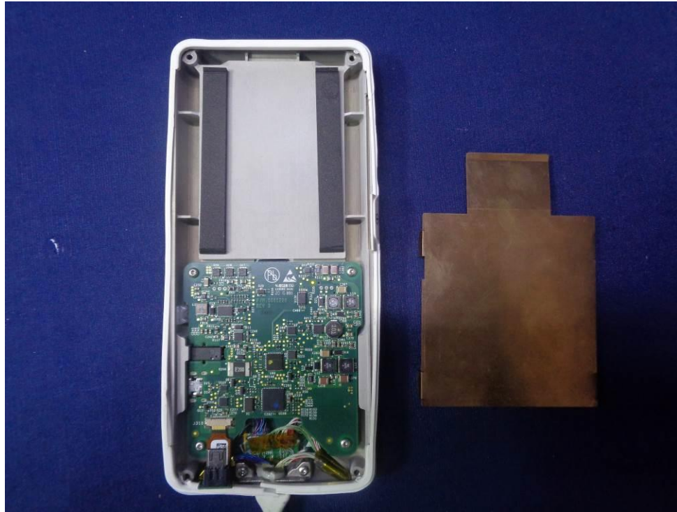
EUT Phone Removed
