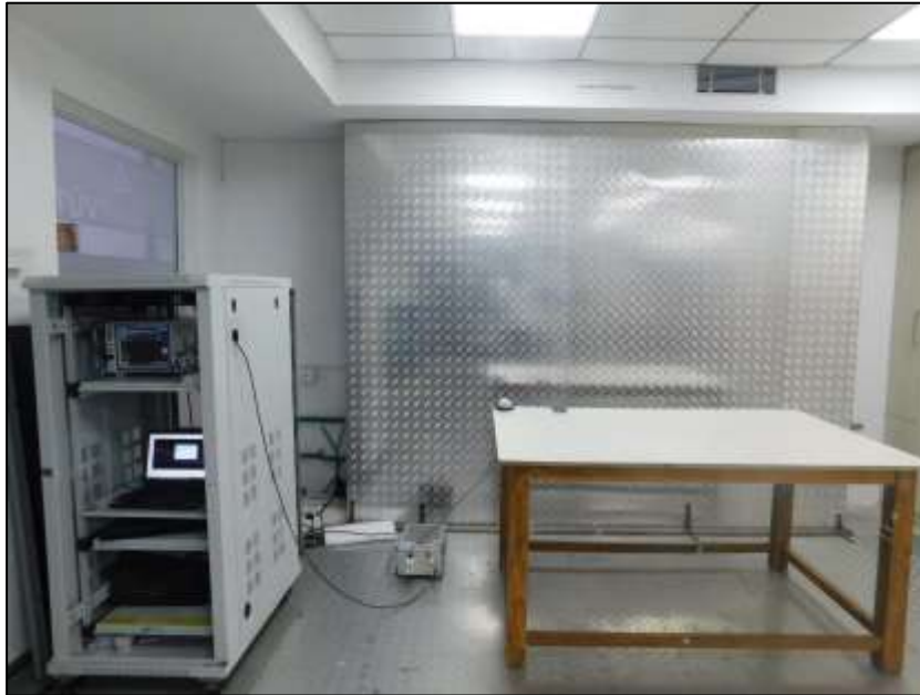
Conducted emission AC power lines test setup with Globe tek Adaptor + Anker charger pad
