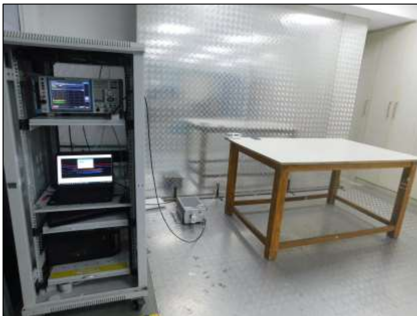
Conducted emission AC power lines test setup with Globe tek Adaptor + Vscan air charger pad
