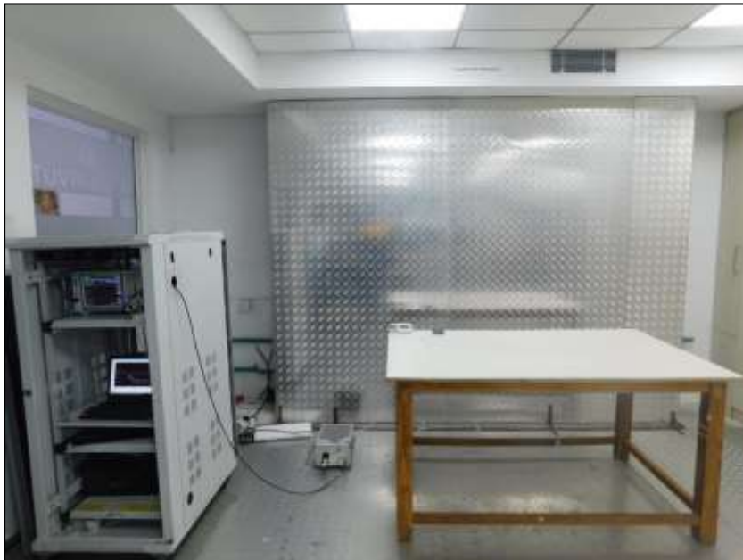
Conducted emission AC power lines test setup with XP Adaptor + Vscan air charger pad
