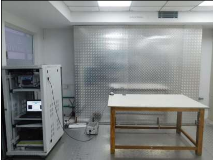
Conducted emission AC power lines test setup with XP Adaptor + Anker charger pad
