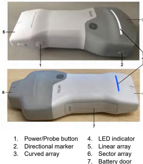
Figure 3-2. Vscan Air probe
