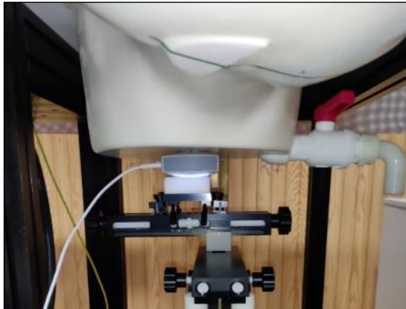
EUT kept in Back position with the flat phantom
