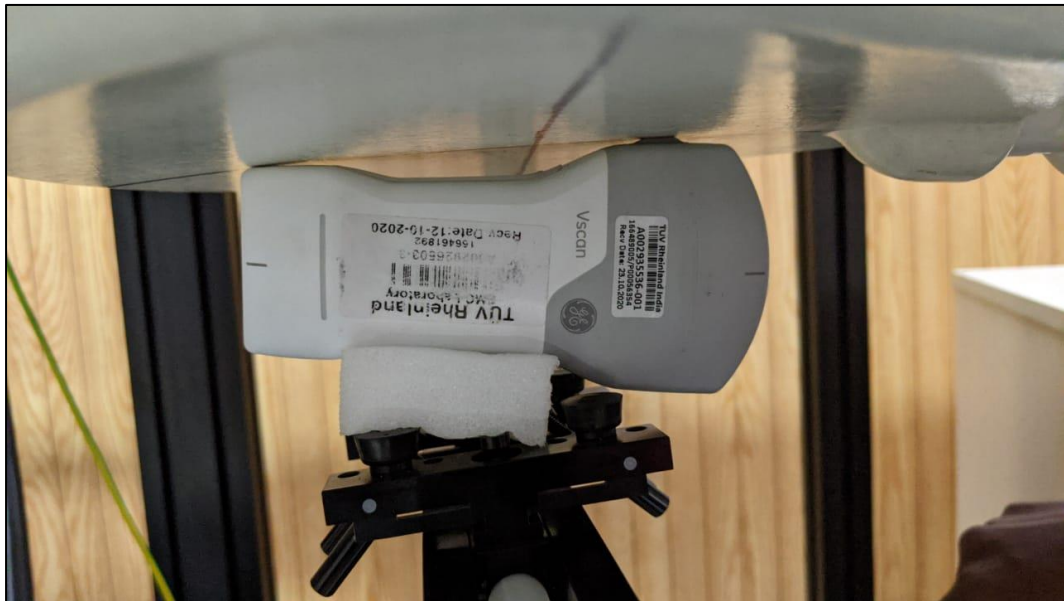
EUT kept in Edge Right position with the flat phantom
