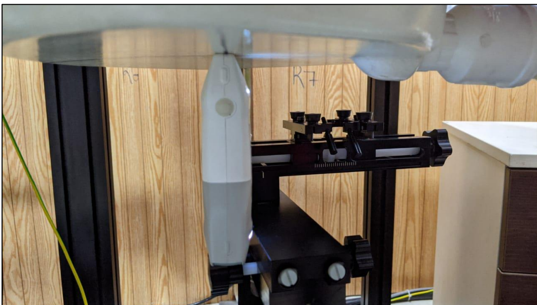
EUT kept in Edge Bottom position with the flat phantom
