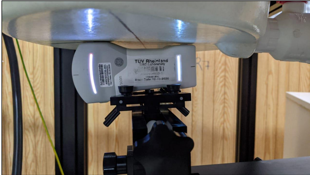
EUT kept in Edge Left position with the flat phantom
