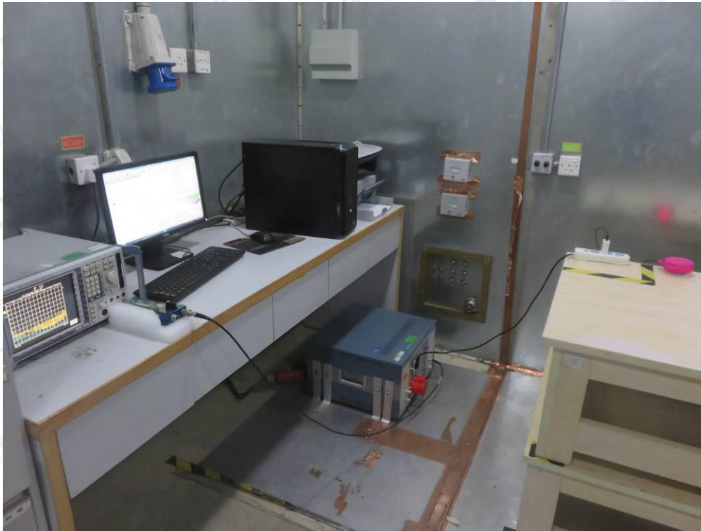
FCC RADIATED EMISSION TEST SETUP
