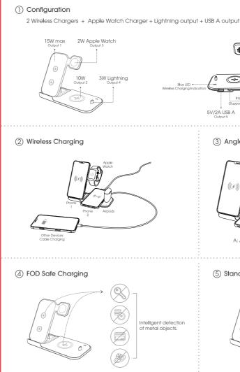
When a foreign object is detected, charging stops and light flashes.
