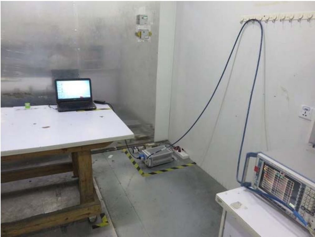
FCC RADIATED EMISSION TEST SETUP
