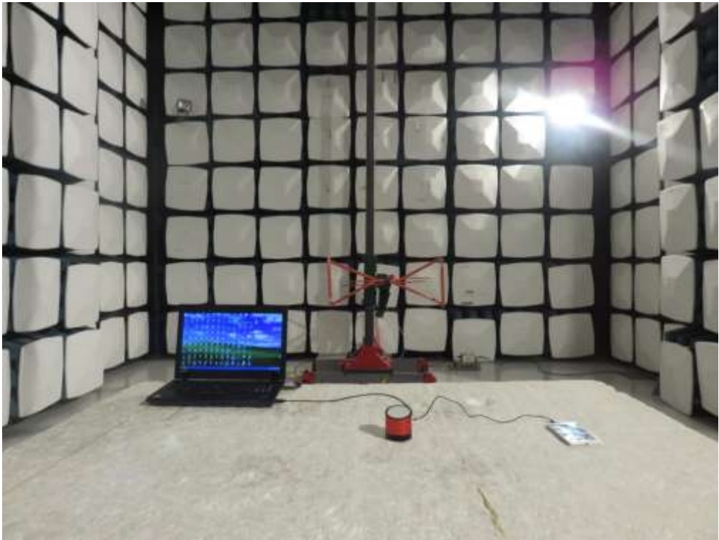
FCC RADIATED EMISSION TEST SETUP
