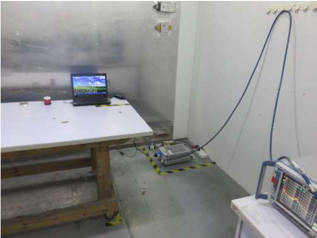
FCC RADIATED EMISSION TEST SETUP
