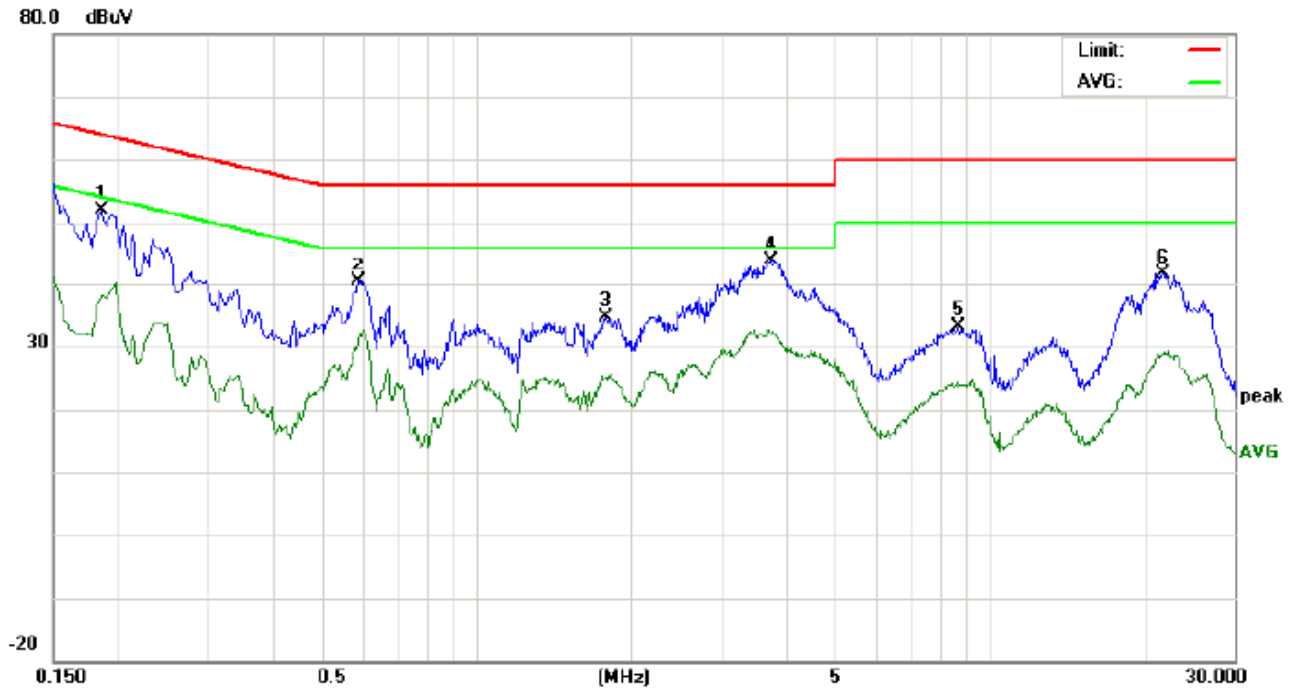
Line Conducted Emission Test Line 1-L
