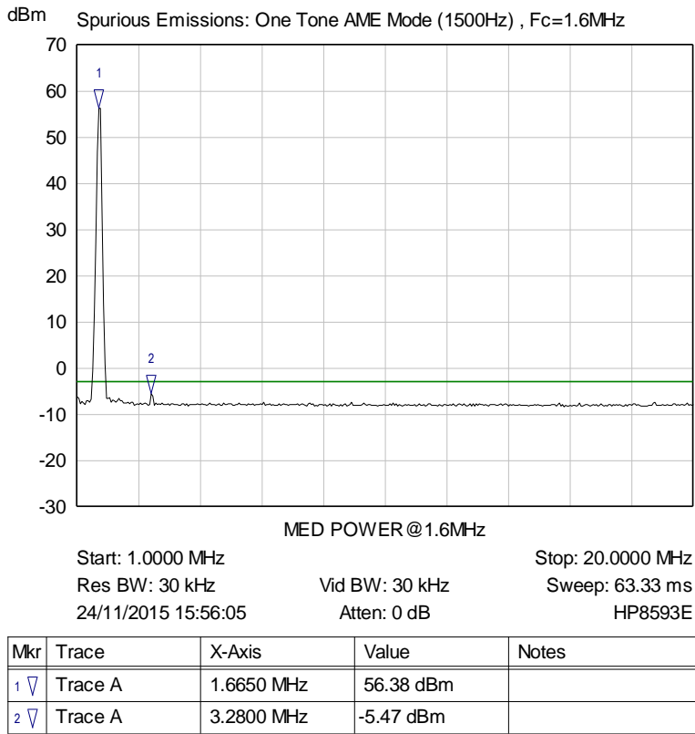
Plot Spurious Emissions at Antenna Terminal; AME Tx=1.6 MHz; P=Med/ 21
