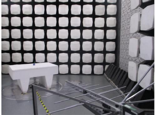
1.2 Radiated Emissions Test Setup (abvoe 1GHz)
