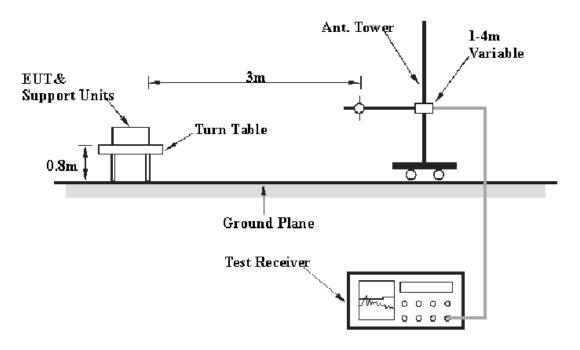
The radiated emission tests were performed in the chamber test site, using the setup accordance with the ANSI C63.4-2009. The specification used was the FCC Part 15 Subpart C, section 15.227 limits.
