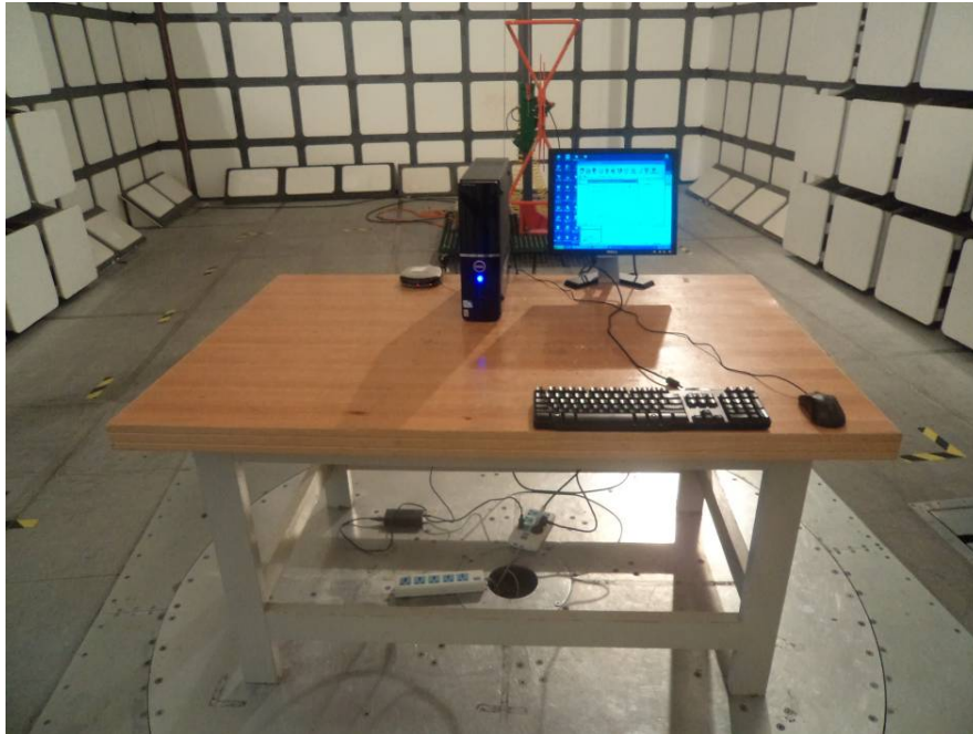
Radiated Emissions – Front View (30-1000 MHz)
