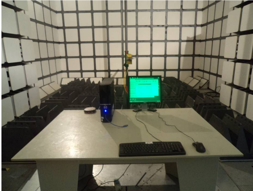
Radiated Emissions – Front View (Above 1 GHz)
