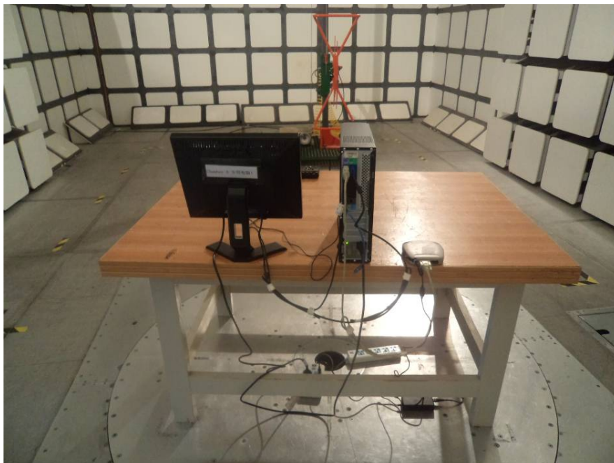
Radiated Emissions – Rear View (30-1000 MHz)
