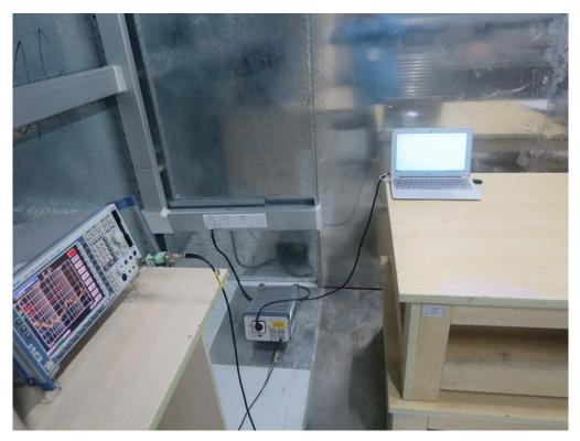
FCC RADIATED EMISSION TEST SETUP
