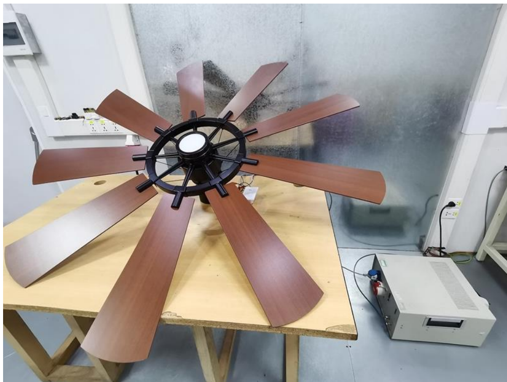
Conducted Emission Test Setup:
