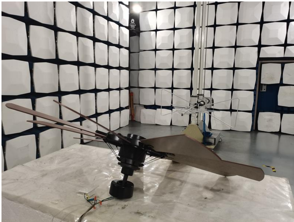
Radiated Emission Test Setup:
