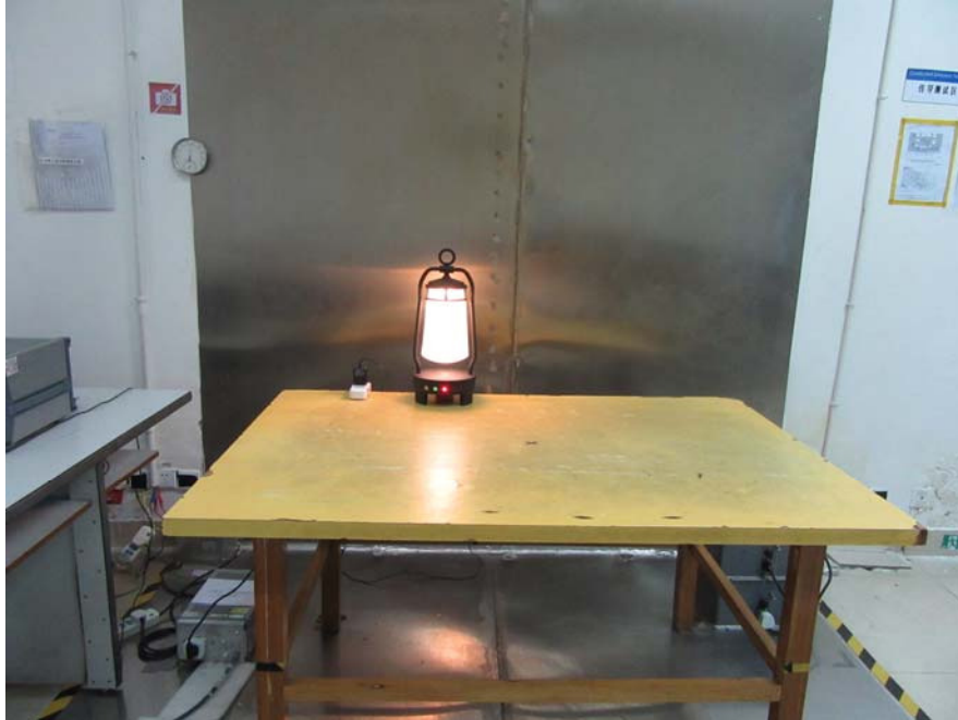
Conducted Emissions – Front View
