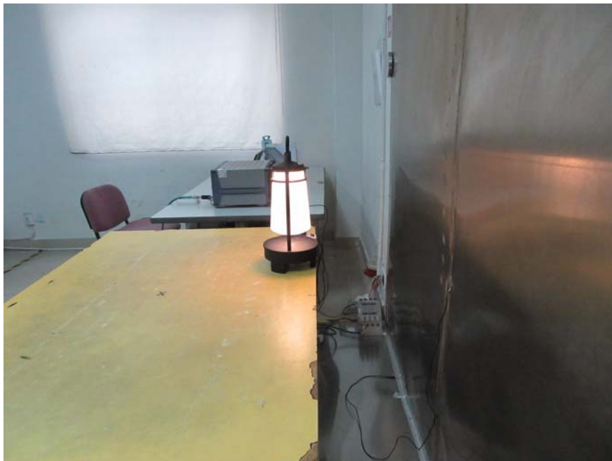
Conducted Emissions – Side View
