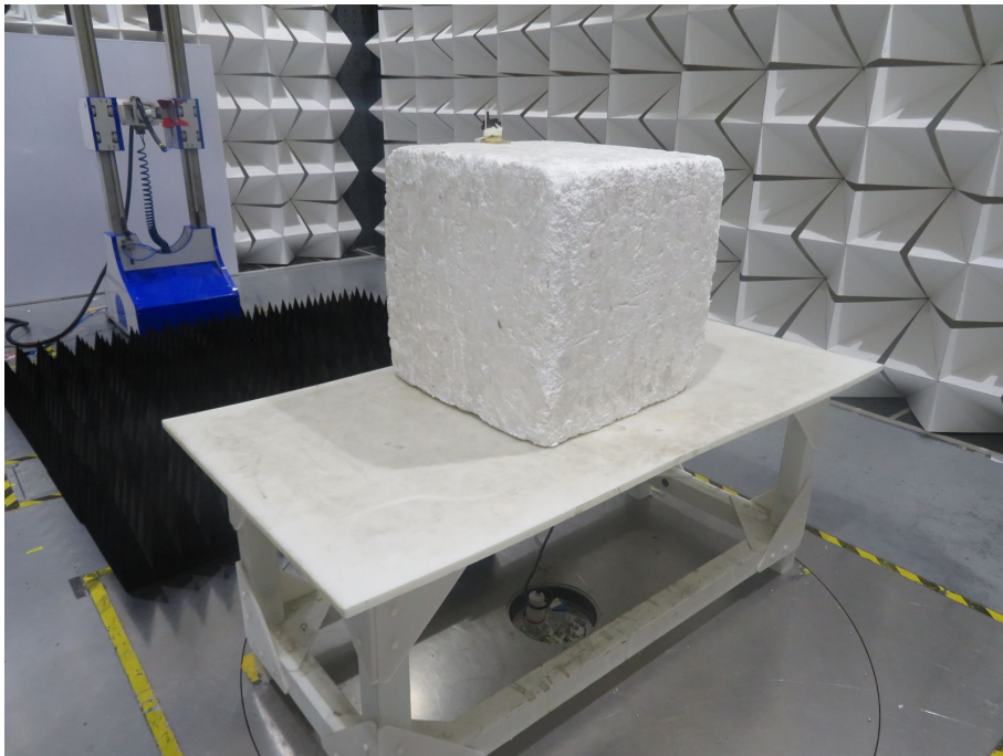
Radiated spurious emission Test Setup-3(Above 1GHz)
