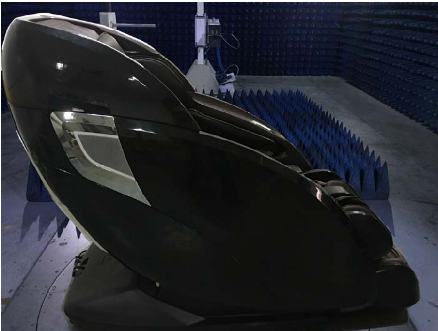
Photograph of set-up for Radiated Emission above 1-18GHz
