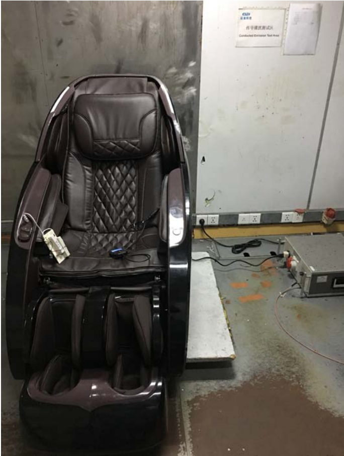
Photograph of set-up for AC Power line Conducted Emission
