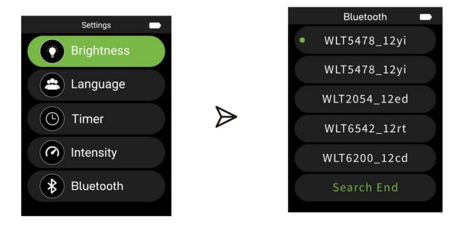
When the product has been installed and powered on, after remote is powered on, you need to select the Bluetooth code of the corresponding control box on the Bluetooth page and press the "ok" button to confirm the connection. then you can start using the product
