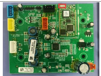
The antenna is Chip antenna. The best case gain of the antenna is 2.5dBi.
