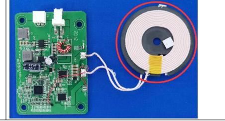
The antenna is Induction coil. The best case gain of the antenna is 0dBi.
