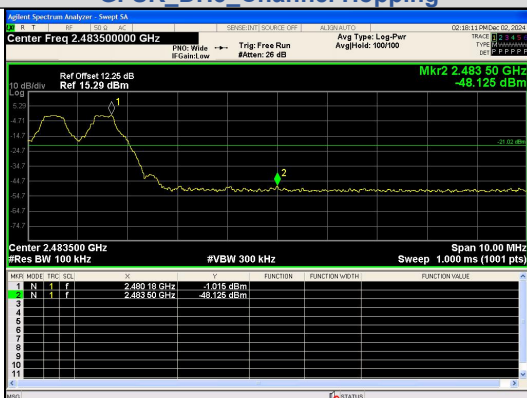
Out Of Band Emission(Right) GFSK_DH5_Channel Hopping
