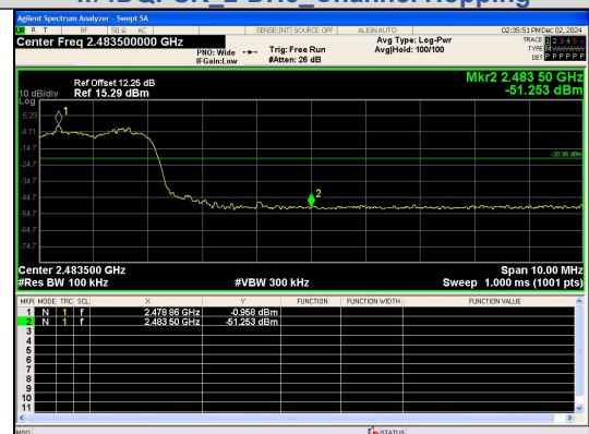
Out Of Band Emission(Right) π/4DQPSK_2-DH5_Channel Hopping
