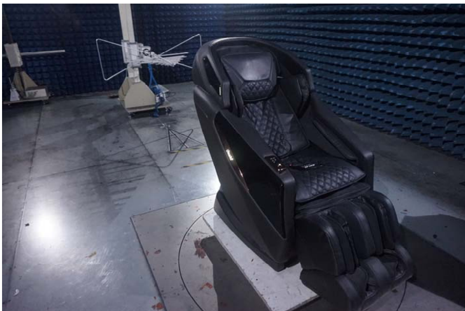
Photograph of set-up for Radiated Emission below 1GHz
