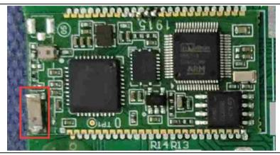
The antenna is Ceramic antenna. The best case gain of the antenna is 2dBi.
