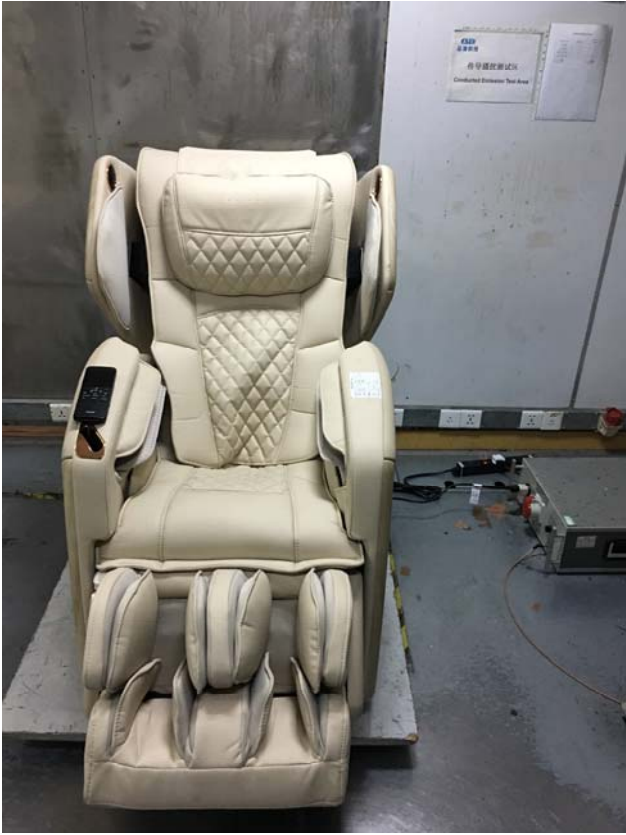
Photograph of set-up for conducted Emission
