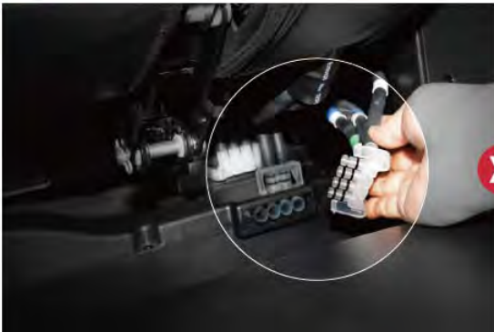
Locate the connector on the inflator pump box.
