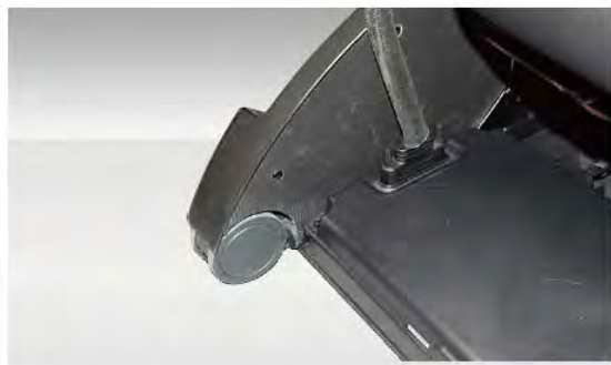
connect the connector to PCB tray. Make sure lock it by the screws.
