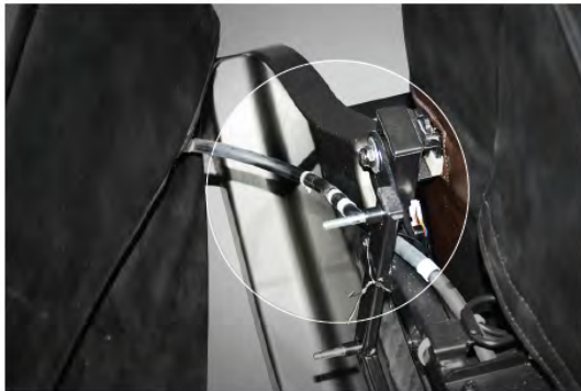
Connect the air hose and wire connectors.
