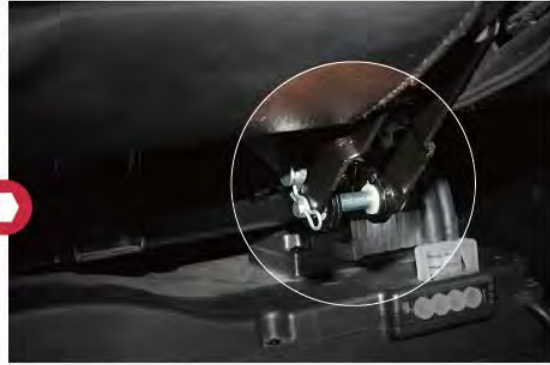
Lock the bolt by cotter pin.
