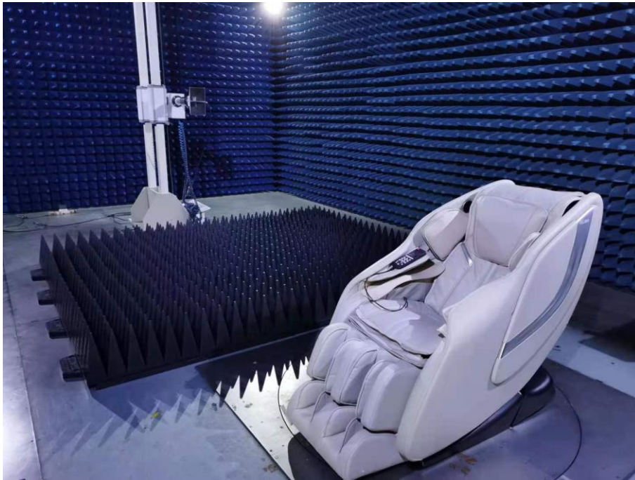
Photo of Radiated Emission Measurement Above 1GHz
