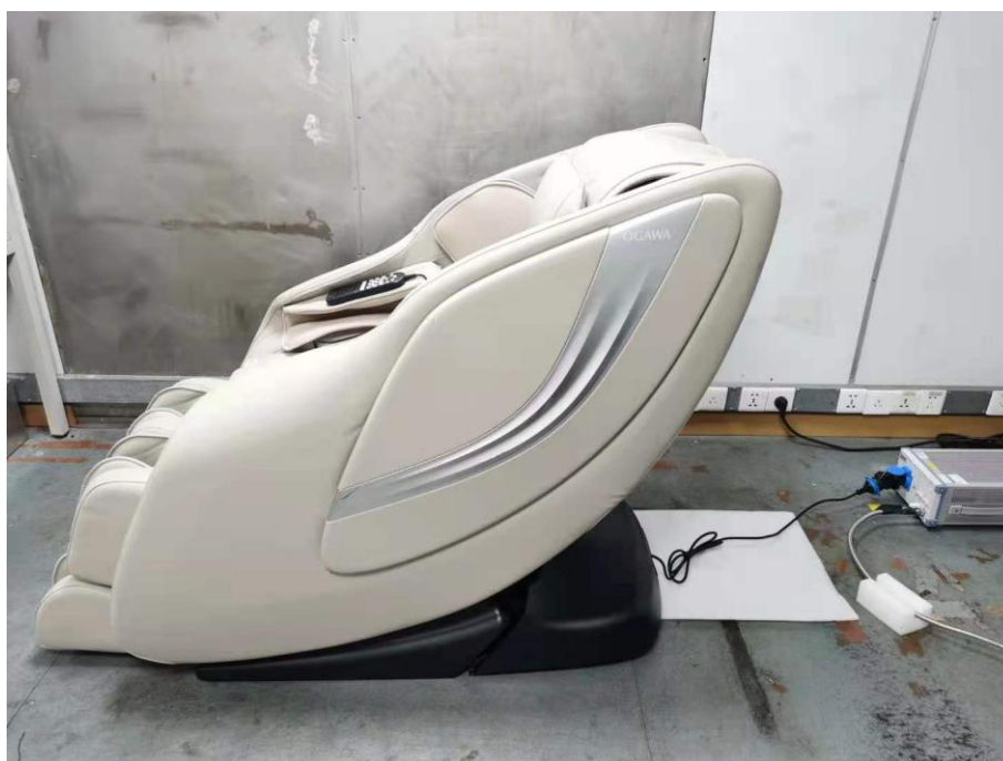
Photo of Power Line Conducted Emission Measurement
