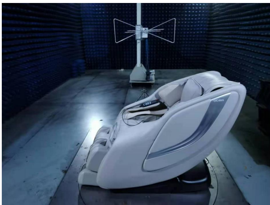
Photo of Radiated Emission Measurement Below 1GHz
