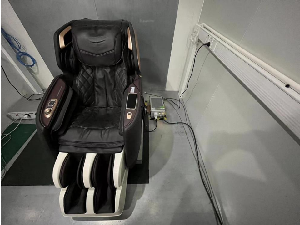
Conducted Emissions Test setup
