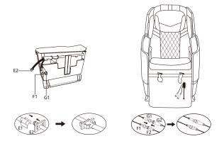
2.Remove the two circlips on the bolts, then attach the footrest onto the base and lock the circlips.
