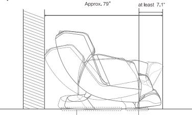
Product's area in contact with the floor. Footrest's area in contact with the floor.
