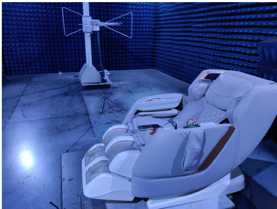
Photo of Radiated Emission Measurement 30MHz - 1GHz
