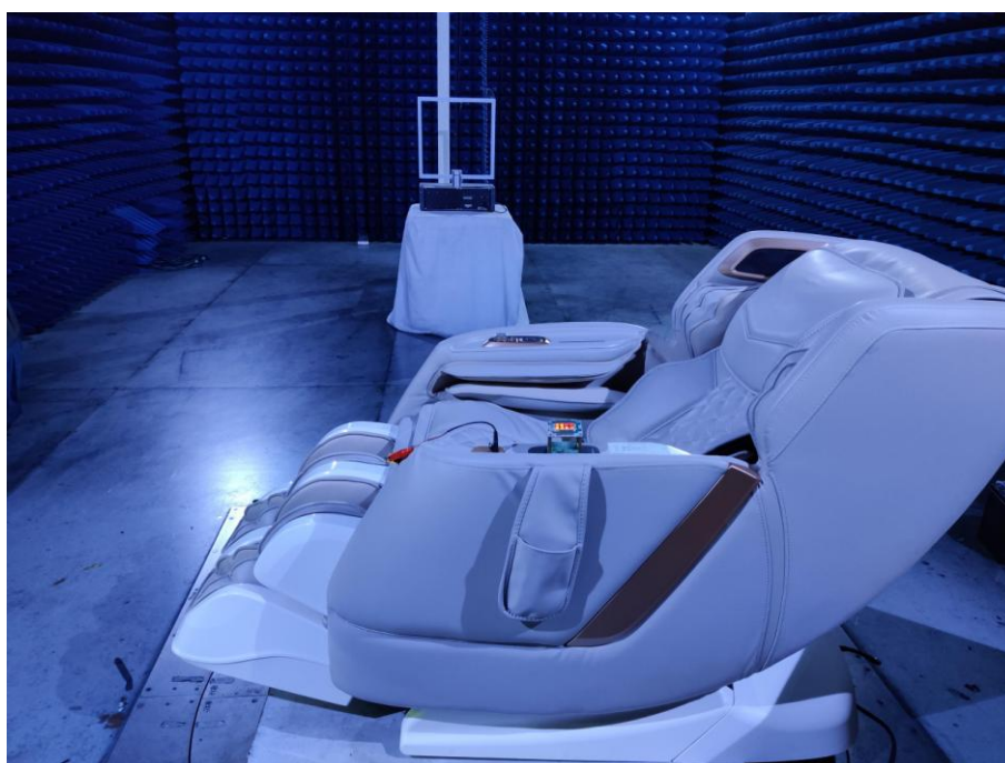
Photo of Radiated Emission Measurement Below 30MHz
