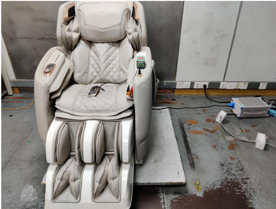
Photo of Power Line Conducted Emission Measurement
