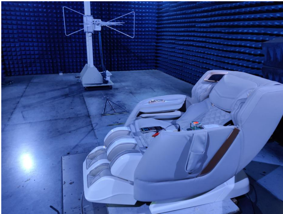
Photo of Radiated Emission Measurement Below 1GHz
