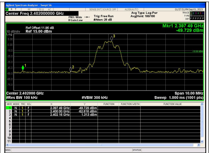
Out Of Band Emission \pi/4 DQPSK_2-DH5_Channel 0
