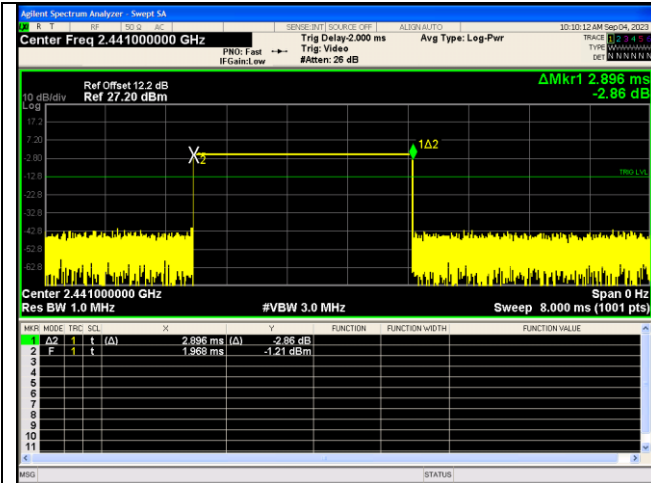
Pulse Width GFSK_DH5
