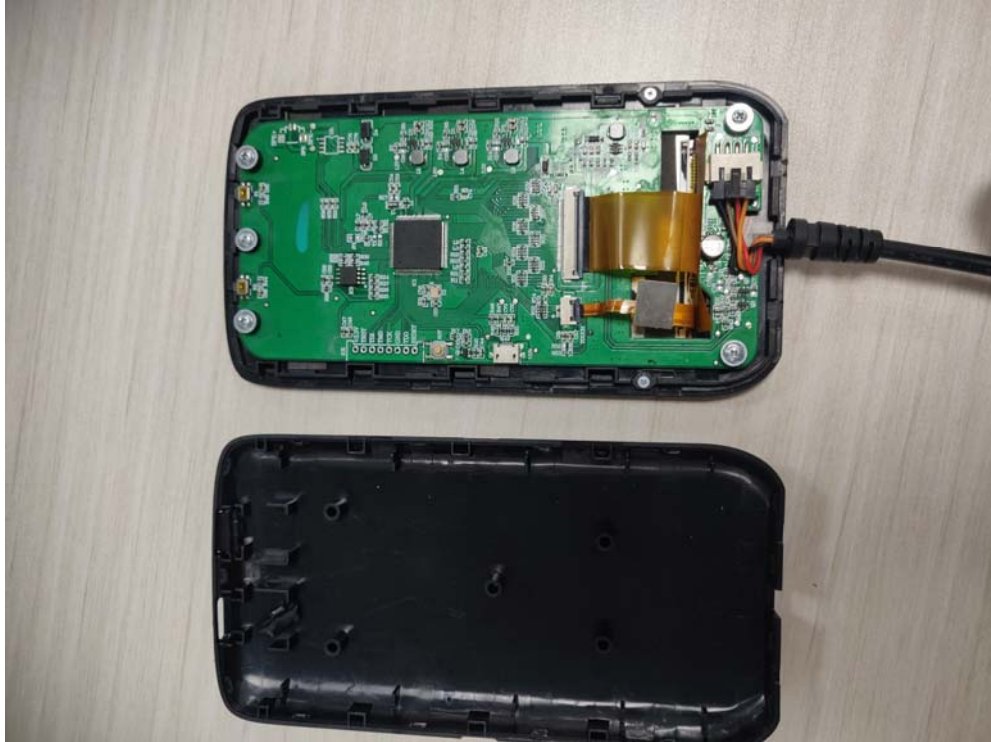
Inside view--Alternative control board
