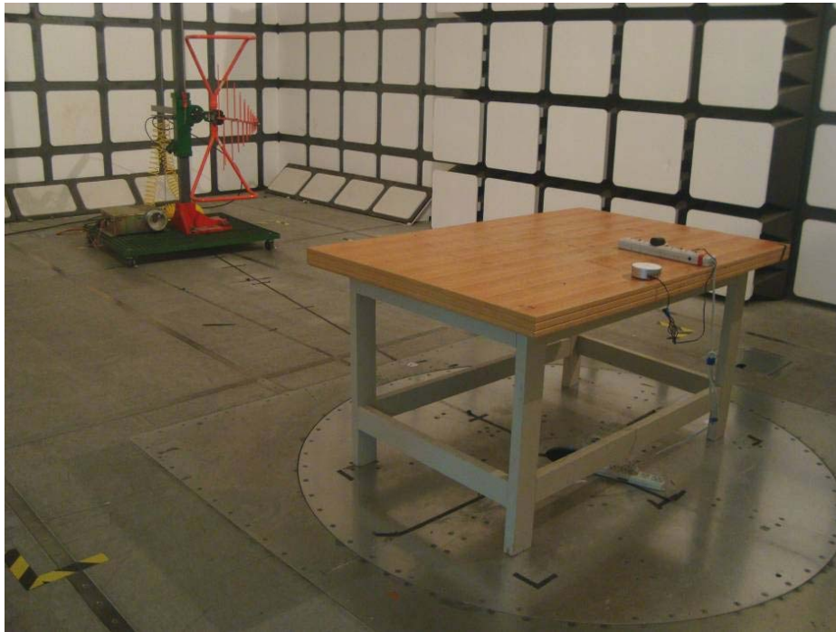
Below 1GHz: Spurious Radiated Emissions - Rear View (with AC/DC adapter)
