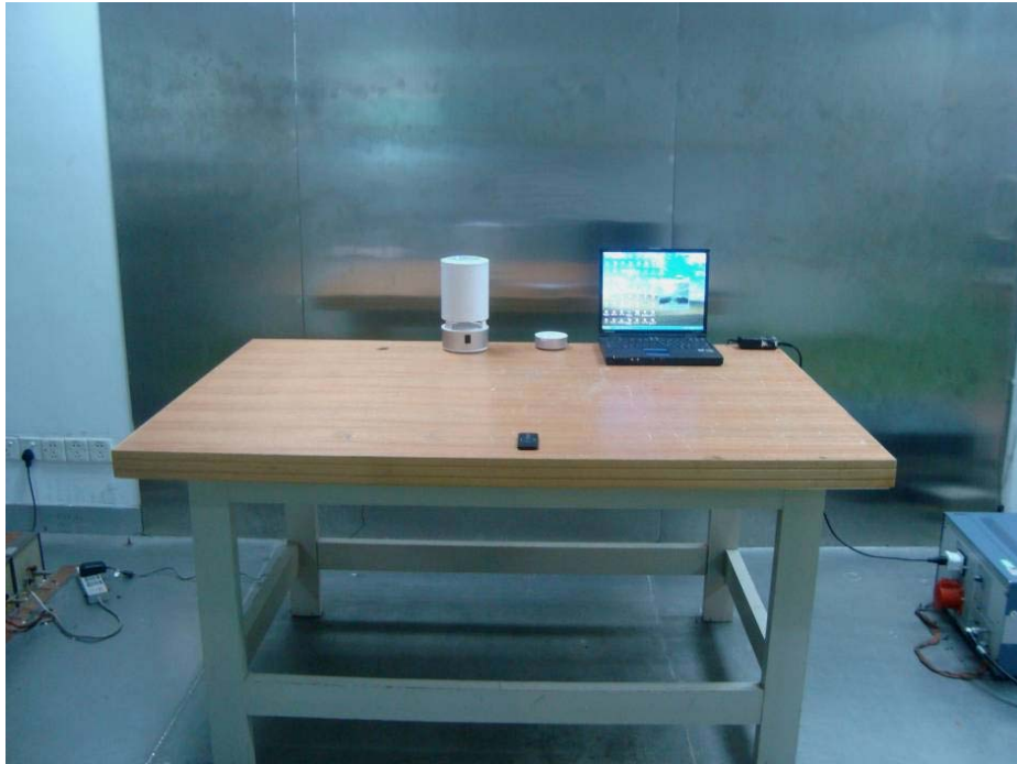
Conducted Emissions - Side View (via USB Port)
