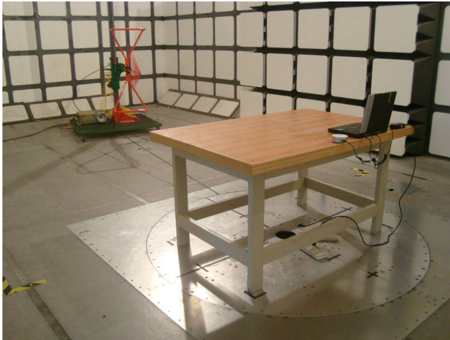
Below 1 GHz: Spurious Radiated Emissions - Rear View (via USB Port)
