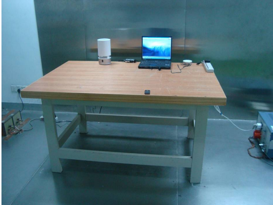
Conducted Emissions - Side View (with AC/DC adapter)
