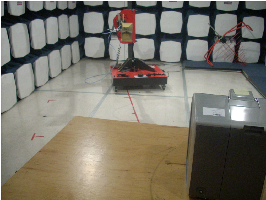
Radiated Spurious Emissions Above 1GHz in Anechoic Chamber
