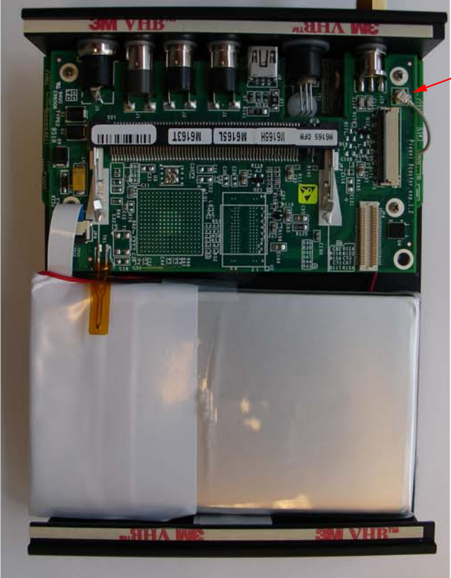
RF connection to main board
