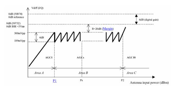
**Area A:** The total gain of the receiver is maximum and constant for all RF input power below P1; the I/Q amplitude increases linearly versus the RF input power until it reaches 300mVpp. The AGC is set to maximum gain AGC1.
