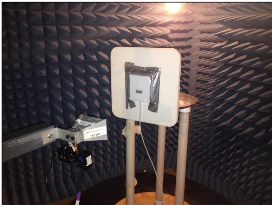
Photograph 5. Radiated Spurs, Test Setup, 18 GHz – 40 GHz, 5 GHz, External Antenna
