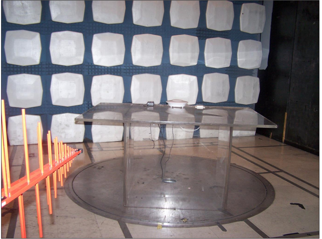
Photograph 2. Radiated Emissions, Test Setup
