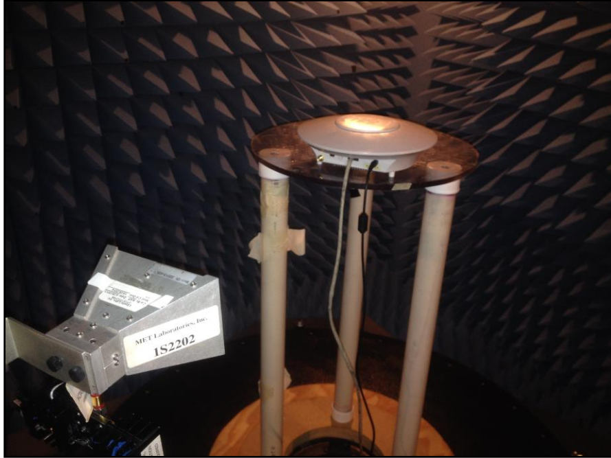
Photograph 8. Radiated Spurs, Test Setup, 18 GHz – 40 GHz, 5 GHz, Internal Antenna
