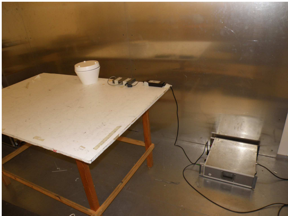
Photograph 1. Conducted emissions at AC power port
