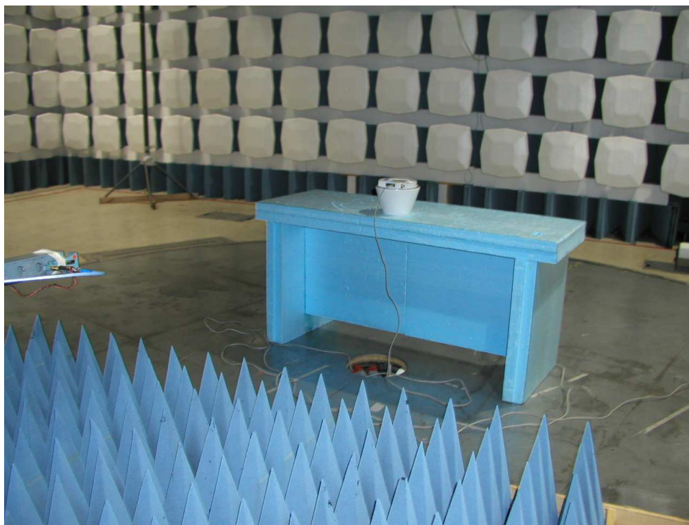
Photograph 2. Radiated emissions measurement
