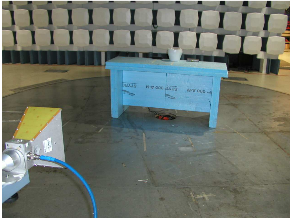
Photograph 2. Radiated emissions test setup
