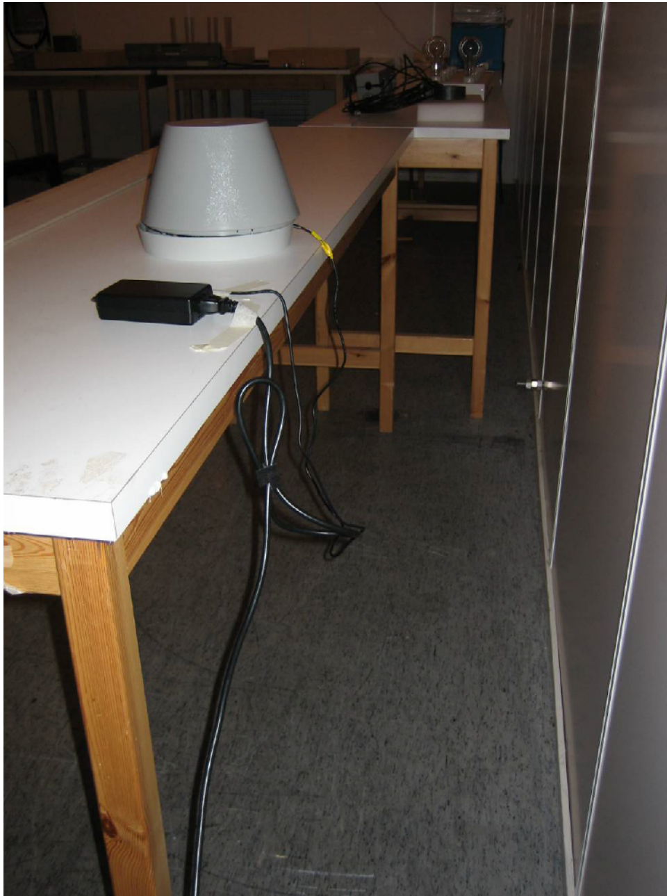
Picture 1. The EUT and test set-up for conducted emission test
