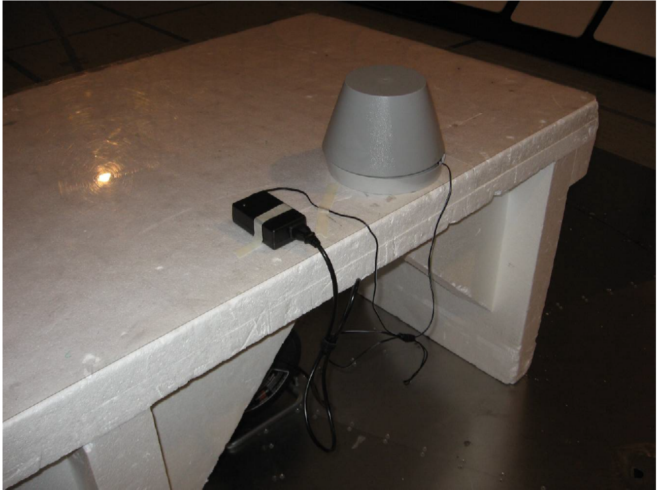
Picture 2. The EUT and test set-up for radiated emission test.
