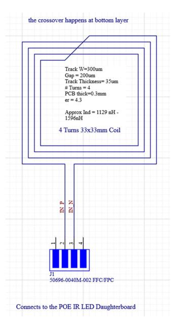
The ADC-VDB755P NFC antenna has a design with the above parameters. The parameters are presented in a graphical way, such that the reader can understand a little bit about it's geometry when reading about it's parameters and characteristics.
