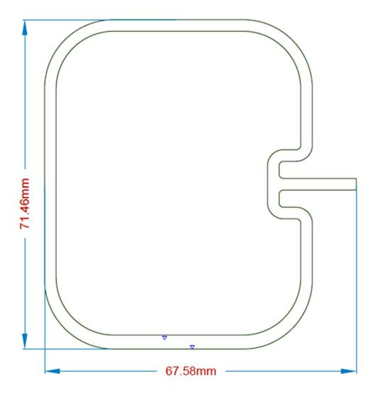
The dimensions of the NFC antenna are as above
