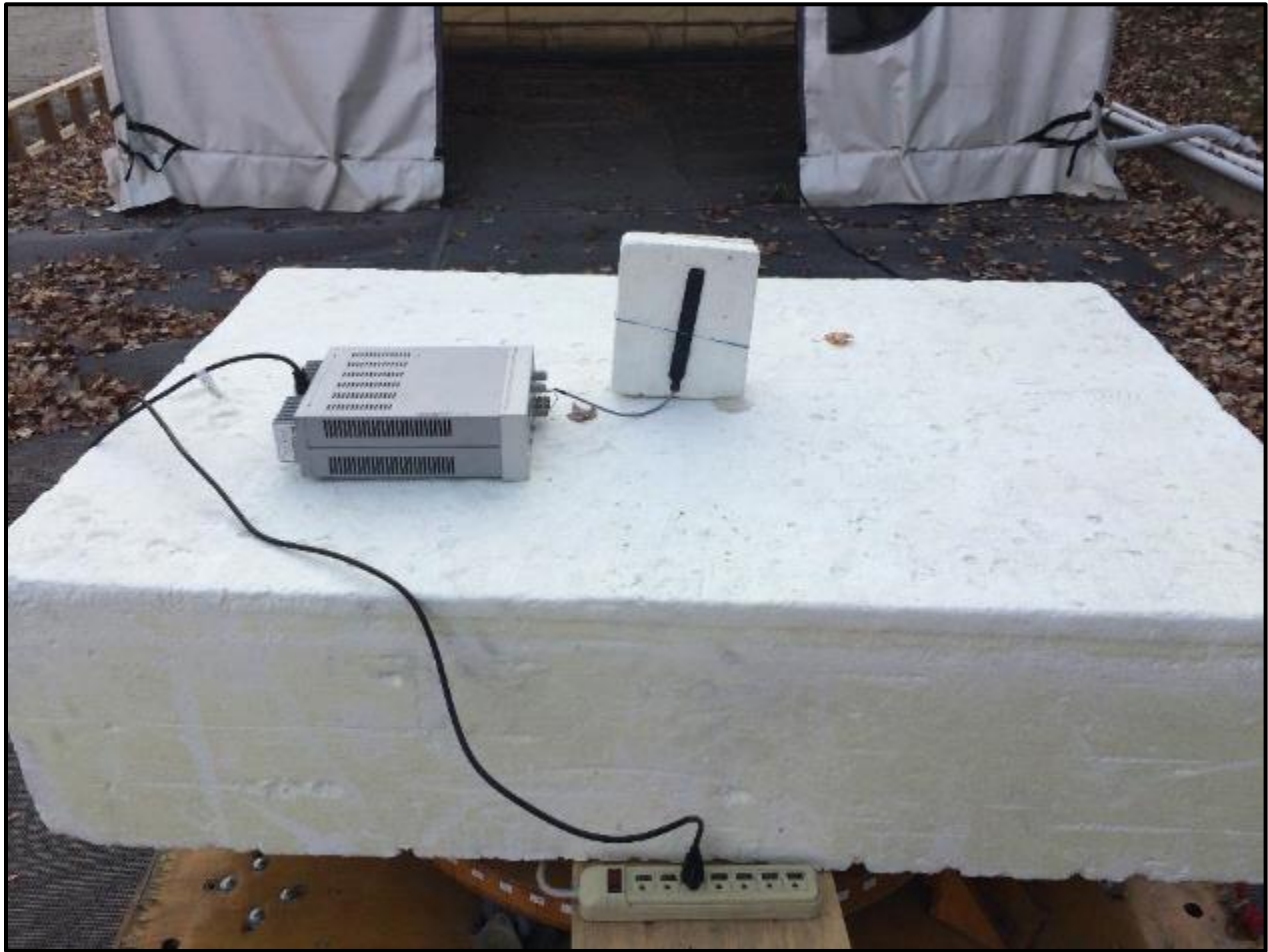
Photograph 3: Radiated Emissions Testing (Digital Emissions, <1 GHz)
