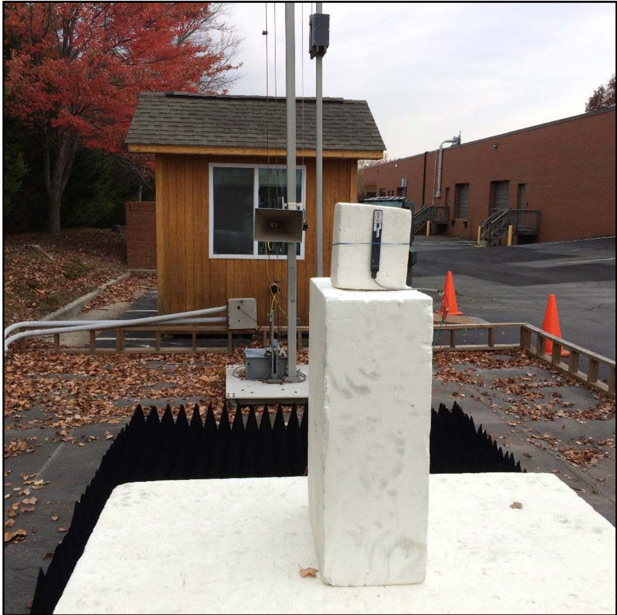
Photograph 4: Radiated Emissions Testing – Front View (Spurious Emissions, >1 GHz)
