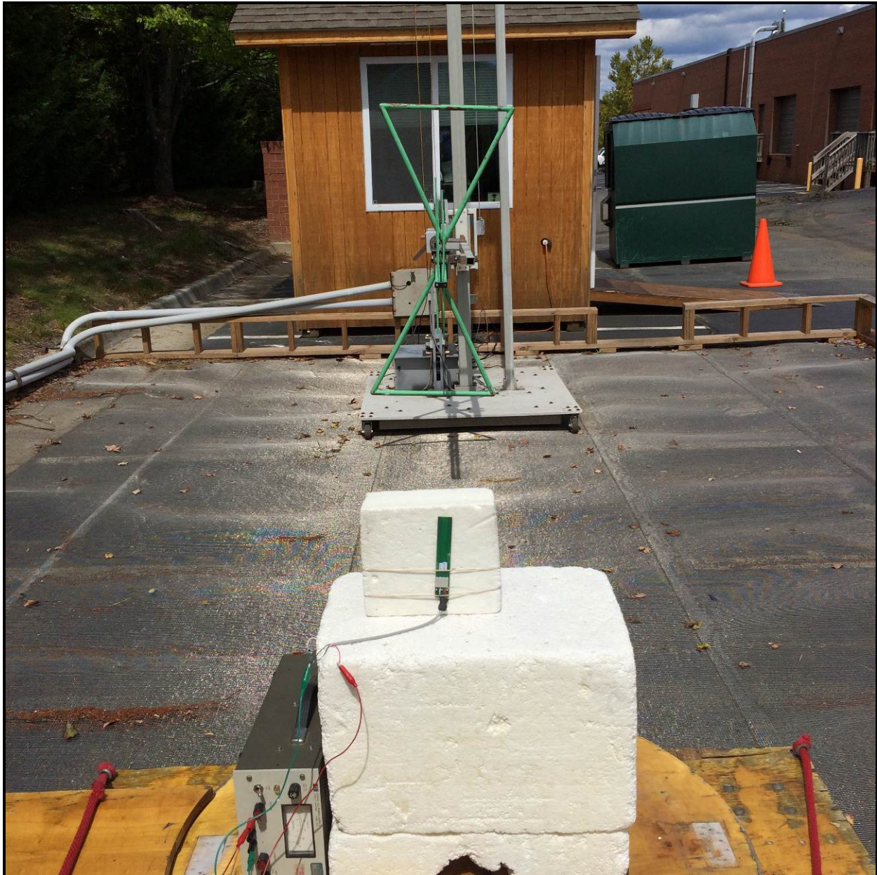
Photograph 3: Radiated Emissions Testing – Front View (Digital Emissions, <1 GHz)
