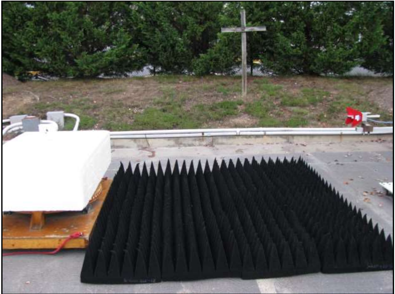
Photograph 5: Radiated Emissions Testing – (Spurious Emissions, >1 GHz)
