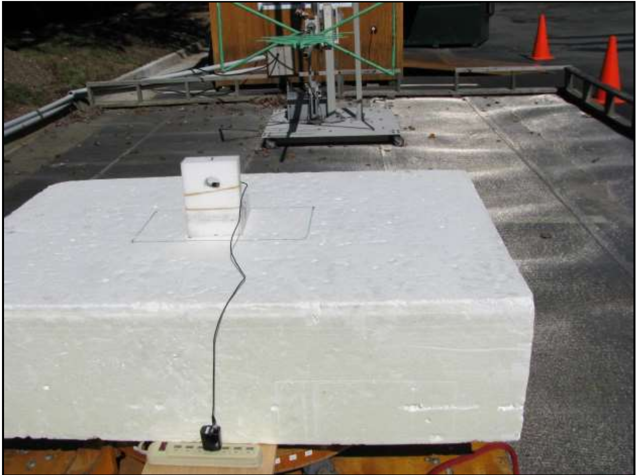
Photograph 3: Radiated Emissions Testing – Back View (Digital Emissions, <1 GHz)
