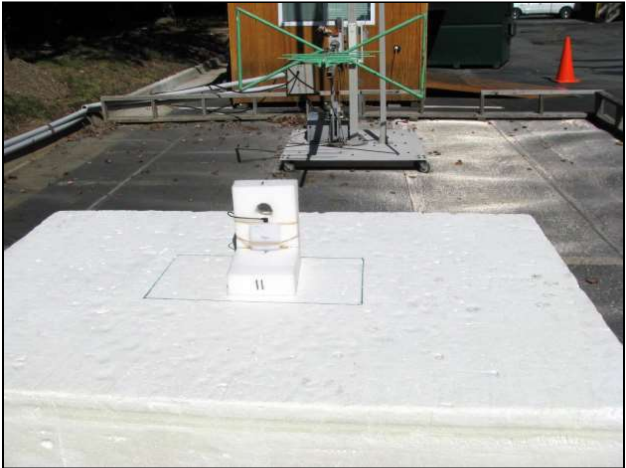
Photograph 2: Radiated Emissions Testing – Front View (Digital Emissions, <1 GHz)
